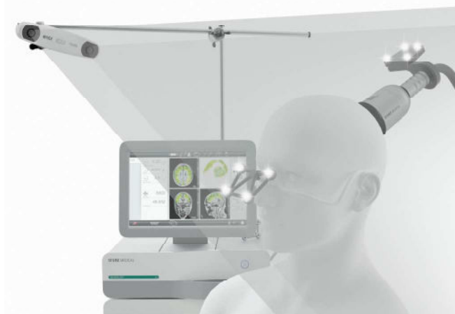
Fig. 4 TPS is administered by a 3-D MRI tracking technique. The position of the stimulation handpiece is detected by a camera which integrates movements of the head. Parameters of the pulses can be adjusted according to the depth and the planned intensity of the stimulation.
